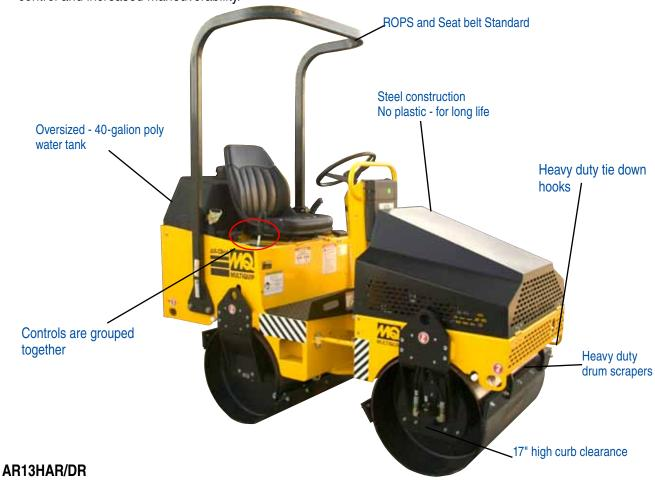
Shown with 20.0-HP (EDA Approved) Honda gas engine\* (manual and recoil start); 23.6 HP Vanguard diesel optional\*
