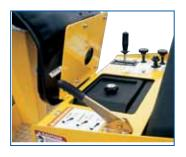
9.5-gal. fuel tank with fuel level indicator cap—located under the seat for easy access. 6.5 hours fuel supply.
