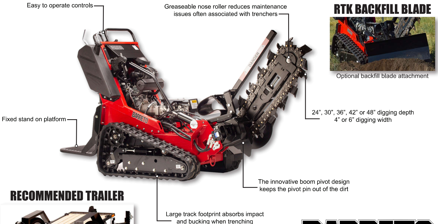
Simple one-handed controls are easy for any operator
